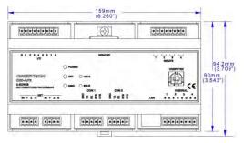
The DIN-AP2 is a 2-Series control processor designed for small to medium-sized lighting and automation applications. DIN Rail mounting enables modular installation alongside Crestron DIN Rail lighting and automation control modules and other third-party DIN Rail mountable devices.
